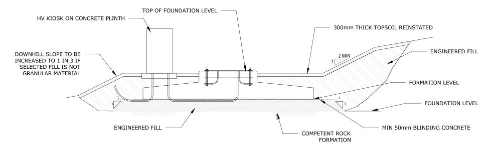
SECTION THROUGH TYPICAL TURBINE BASE
