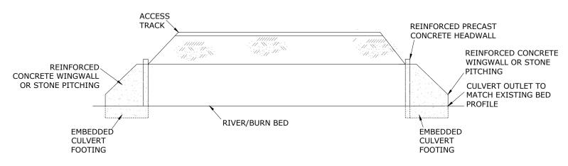
TYPICAL CROSS SECTION THROUGH CULVERT (NTS)
