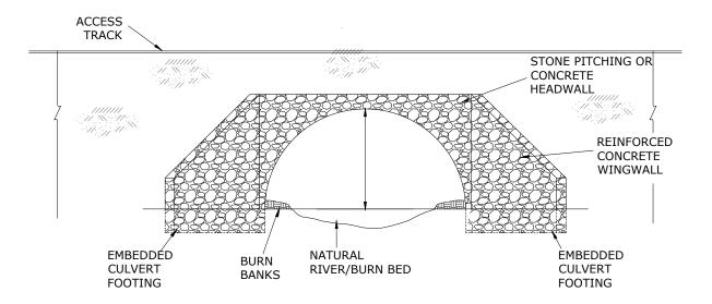
TYPICAL BOTTOMLESS ARCHED CULVERT ELEVATION (NTS)
