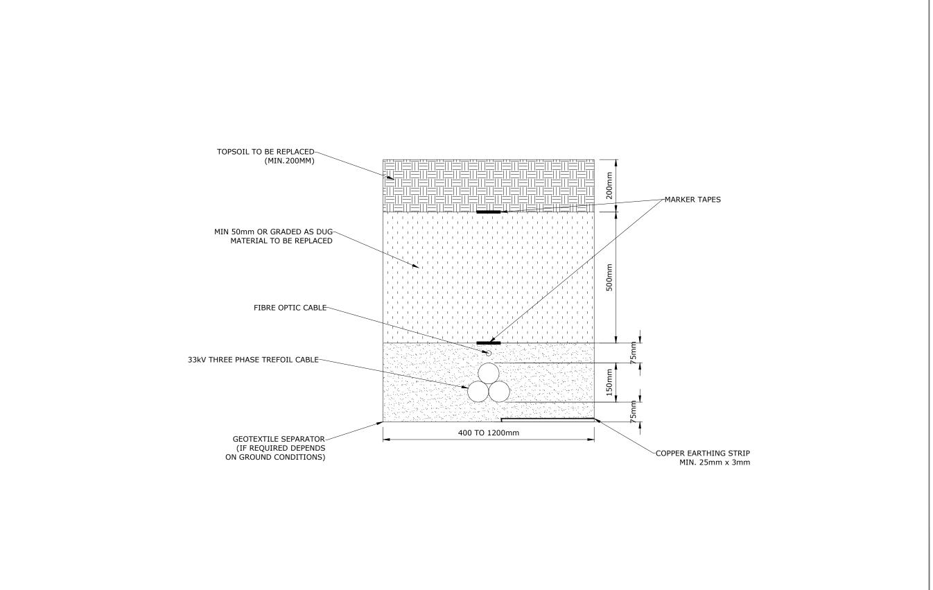
Typical Cable Trench Detail Figure 3.11 Project: Lochluichart Wind Farm Extension II Source:
