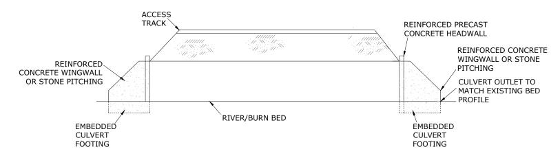
TYPICAL CROSS SECTION THROUGH CULVERT (NTS)
